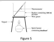
"Mass of spirit burner and fuel before combustion ------ 234.00 grams Mass of spirit burner and fuel after combustion ------ 231.69 grams Temperature of water before combustion ------ 25.0 °C Temperature of water after combustion ------ 69.2 °C
